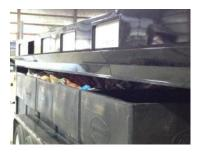
Refurbishment of residential recycling trailers and the addition of modified corrugated cardboard containers have resulted in improved efficiencies. The trailers can now be easily emptied without the threat of injury to employees (as was the case with the old faulty lid design).
